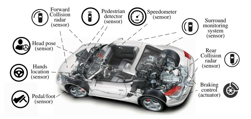
Maneuver Assistance System (MAS) is expected to increase the driver's safety by monitoring its behaviour, detecting unintended maneuvers, and respond in a way that guarantees the highest possible level of driver safety.
