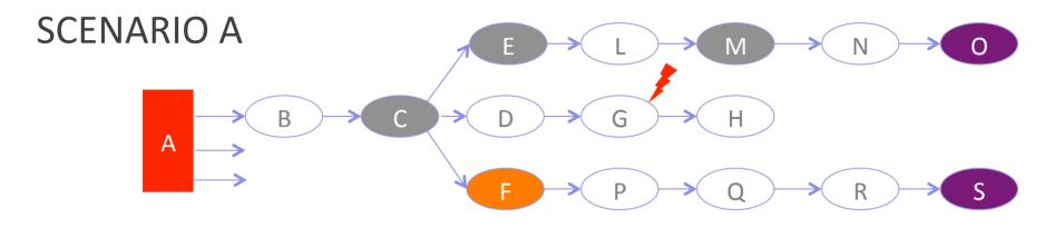
T=0 Severe failure on SS G T=0 All nodes on line will be disconnected
