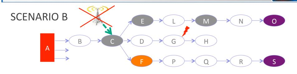
T=0 Severe failure on SS G T=0 All nodes on line will be disconnected
